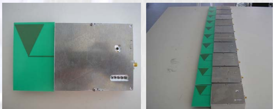
Figure 3. Photo of the antenna/receiver and the whole receiving unit by putting 10 separate receiving modules in a row
