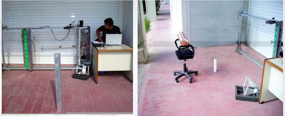
Figure 5. Measurement setup for air and metallic/dielectric objects
